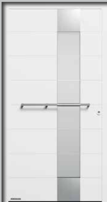
Style 697 Stainless steel handle HOE 910, stainless steel embellishments, matt Parsol grey design glass (single-pane safety glass) with 7 clear stripes, triple thermal insulation glass, U_D -value up to approx. 0.9 \text{ W}/(\text{m}^2\cdot\text{K})^*
